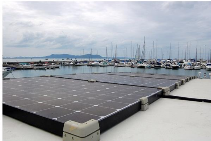
The 12-solar panels on the roof of the refitted catamaran
